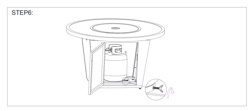
Place propane gas tank (not included) into the cylinder base (G).Make sure the gas tank sits on the cylinder base (G) completely. Turn the preassembled wing screw on the outer part of cylinder base (G) clockwise to secure the propane gas tank tightly.
