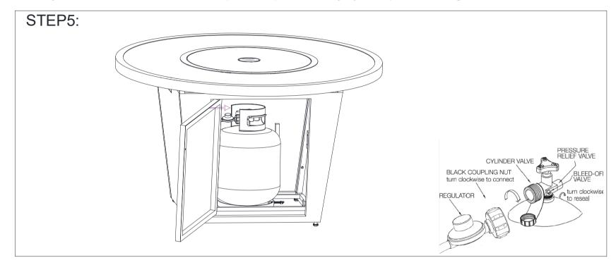
Turn the cylinder valve on the tank clockwise to close the propane tank. Attach the pre-assembled regulator from the table top (B) to the cylinder valve by turning the regulator coupling nut clockwise. Make sure it is fastened securely and tighten connections by hand only.
