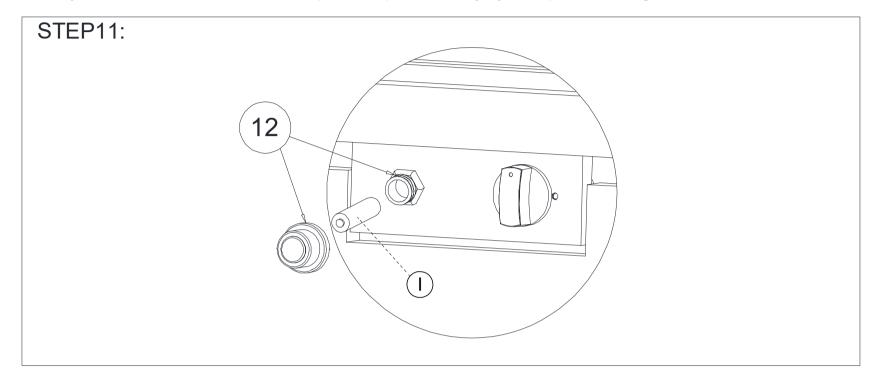
Remove the rubber cap on the electronic igniter (12) by unscrewing and slide battery into the battery slot. Make sure the positive side of the battery faces outwards. Screw the electronic igniter cap (12) over the battery tightly. The ignition module requires one Alkaline AA size battery (1.5V).
