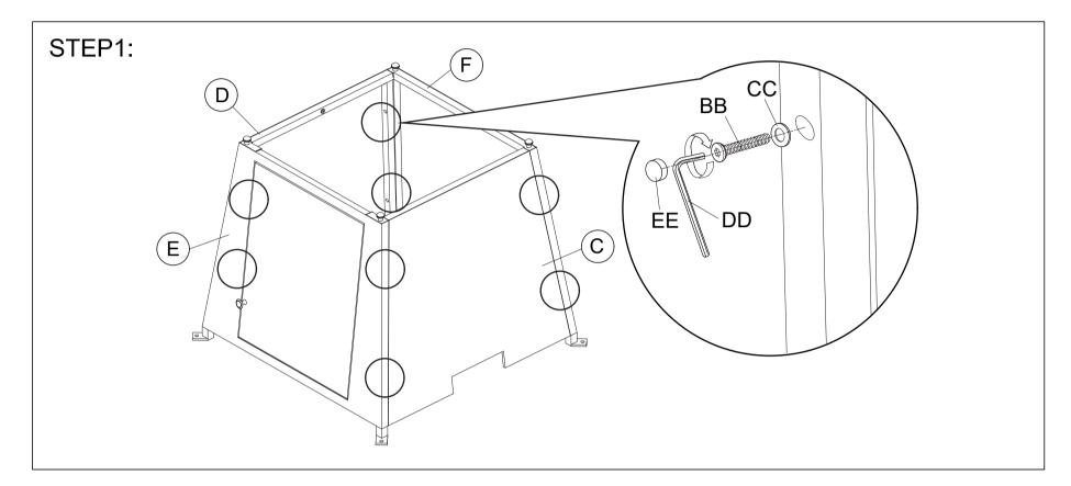
Attach the right side panel(C) and left side panel(D) to the firepit door(E) and back side banel(F) with bolts and washers.
