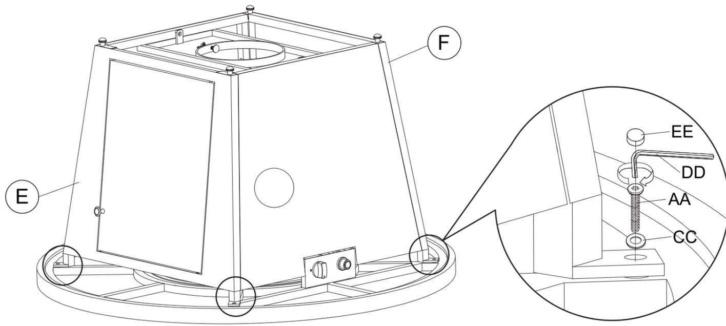
Attach the firepit door(E) and back side panel(F) to the table top(B) with bolts and washers.
