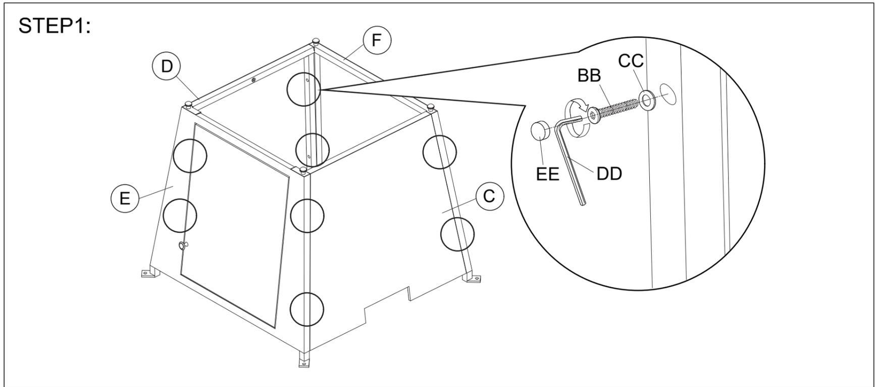
Attach the right side panel(C) and left side panel(D) to the firepit door(E) and back side panel(F) with bolts and washers.
