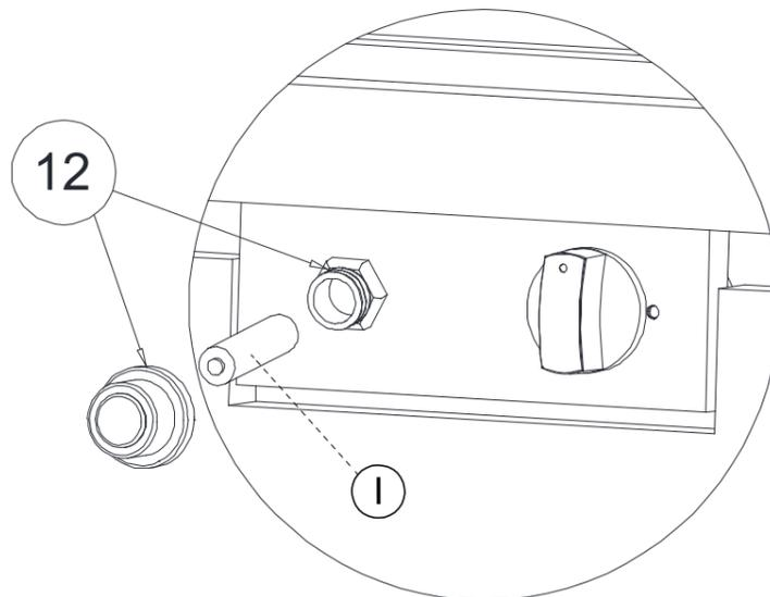
Remove the rubber cap on the electronic igniter ( 12 ) by unscrewing and slide battery into the battery slot. Make sure the positive side of the battery faces outwards. Screw the electronic igniter cap ( 12 ) over the battery tightly. The ignition module requires one Alkaline AA size battery (1.5V).
