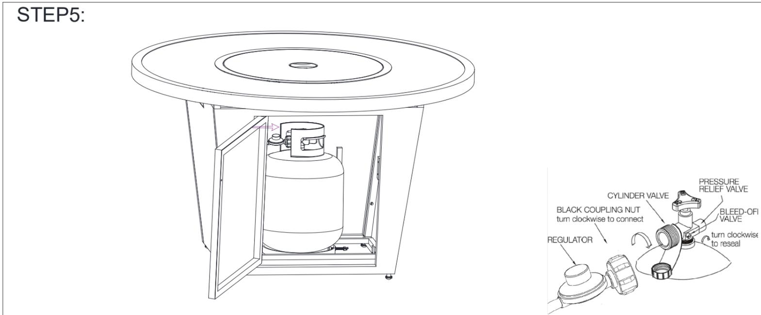
Turn the cylinder valve on the tank clockwise to close the propane tank. Attach the pre-assembled regulator from the table top ( B ) to the cylinder valve by turning the regulator coupling nut clockwise. Make sure it is fastened securely and tighten connections by hand only.
