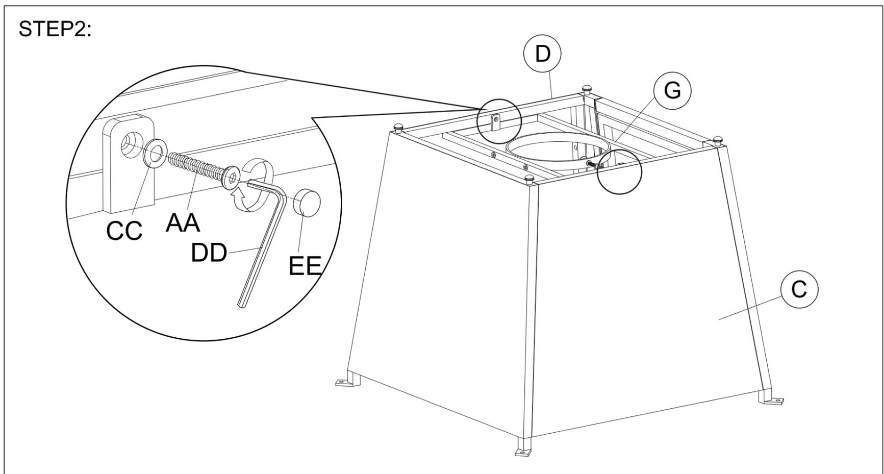
Attach the gas cylinder holder(G) to the right side panel(C) and left side panel(D) with bolts and washers.
