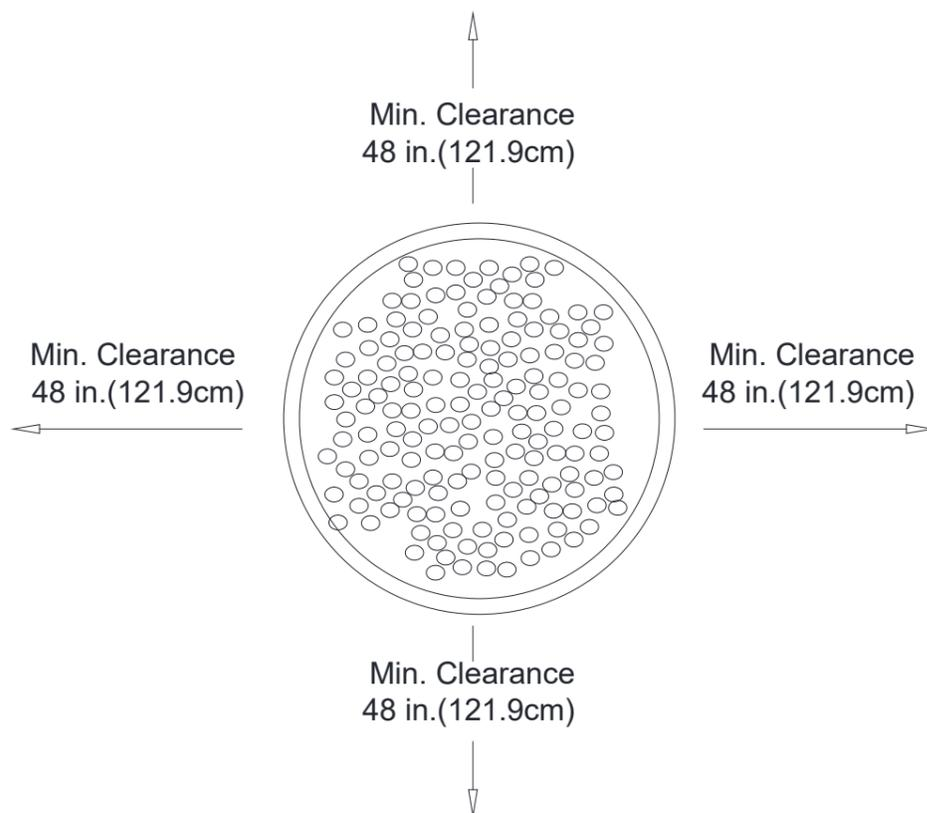
Combustible materials should not be within 60 inches of the top of the unit, or within 48 inches around the entire unit.
