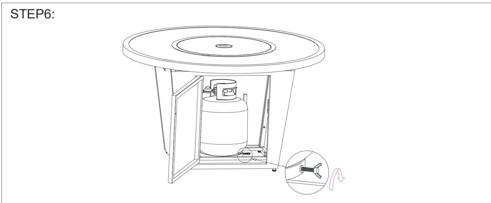
Place propane gas tank ( not included ) into the cylinder base ( G ). Make sure the gas tank sits on the cylinder base ( G ) completely. Turn the preassembled wing screw on the outer part of cylinder base ( G ) clockwise to secure the propane gas tank tightly.
