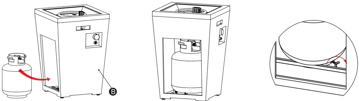
3 Place propane tank (not included) in the metal stand inside Body (B) and make sure the gas tank sits on the metal stand completely. Turn the wing screw on the outer part of metal stand clockwise to secure the gas tank tightly.
