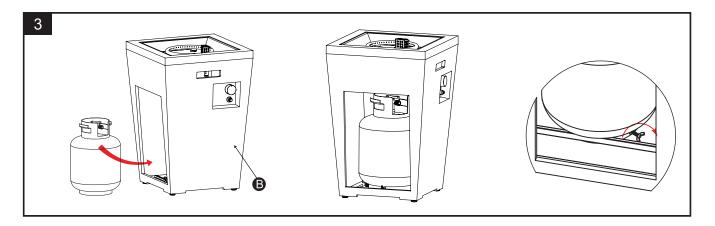
**3** Place propane tank (not included) in the metal stand inside Body (B) and make sure the gas tank sits on the metal stand completely. Turn the wing screw on the outer part of metal stand clockwise to secure the gas tank tightly.
