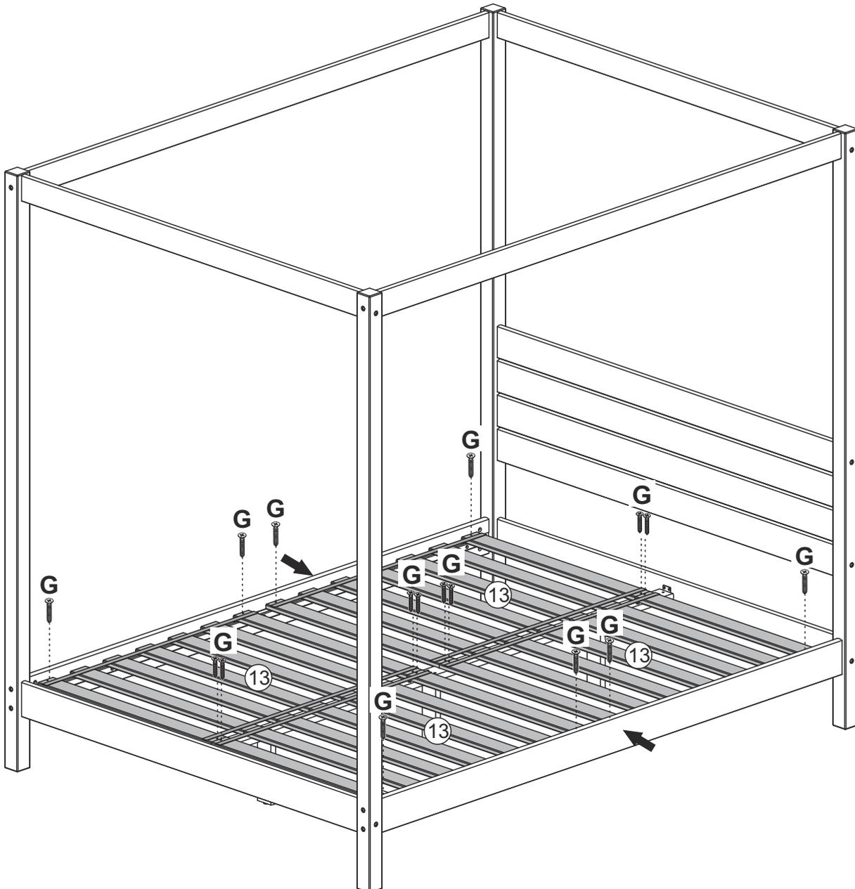
Secure the set of slats 18 with screw (G) using phillips head screwdriver.
