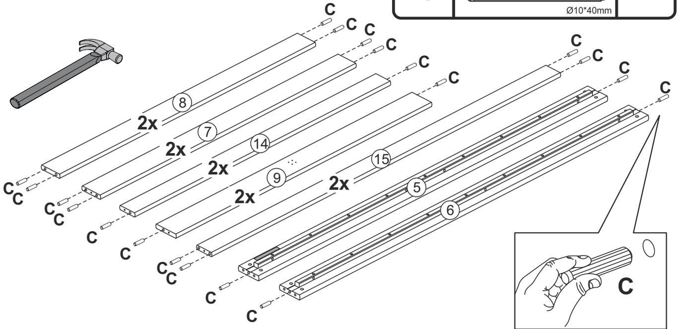
Insert wood dowel (C) into parts (5,6,7,8,9,14 and (15).
