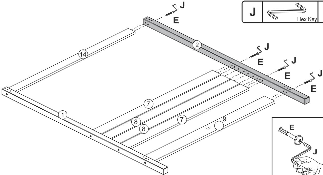
Secure part 2 to parts 7, 8, 9 and 14 with screw (E) using Hex Key (J).
