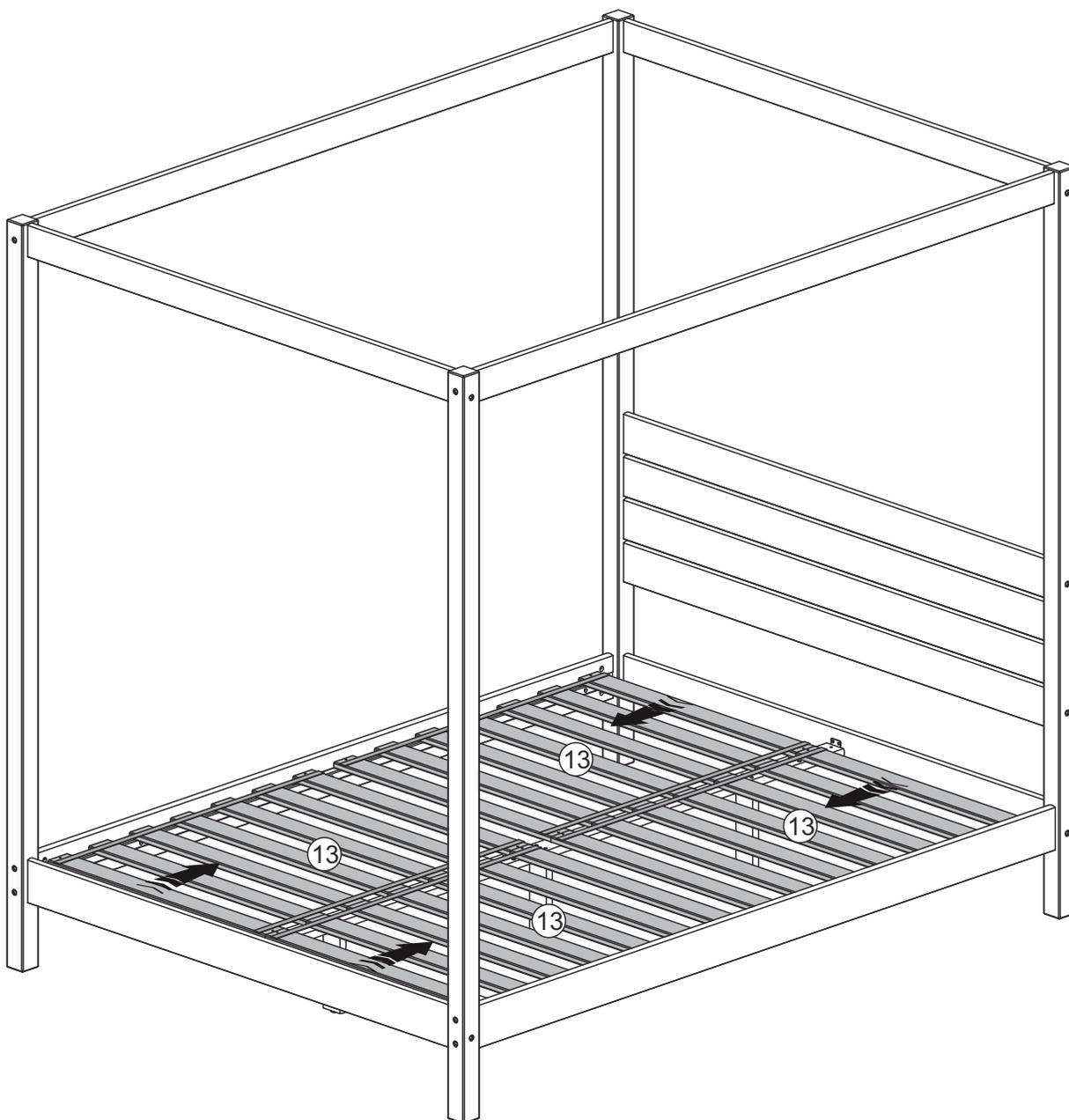
Insert the set of slats 13 as shown in the diagram.
