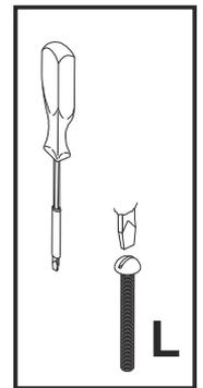
Secure part 11 to support (K) with screw (L) and washer (N) and nut (M) using slotted head screwdriver.
