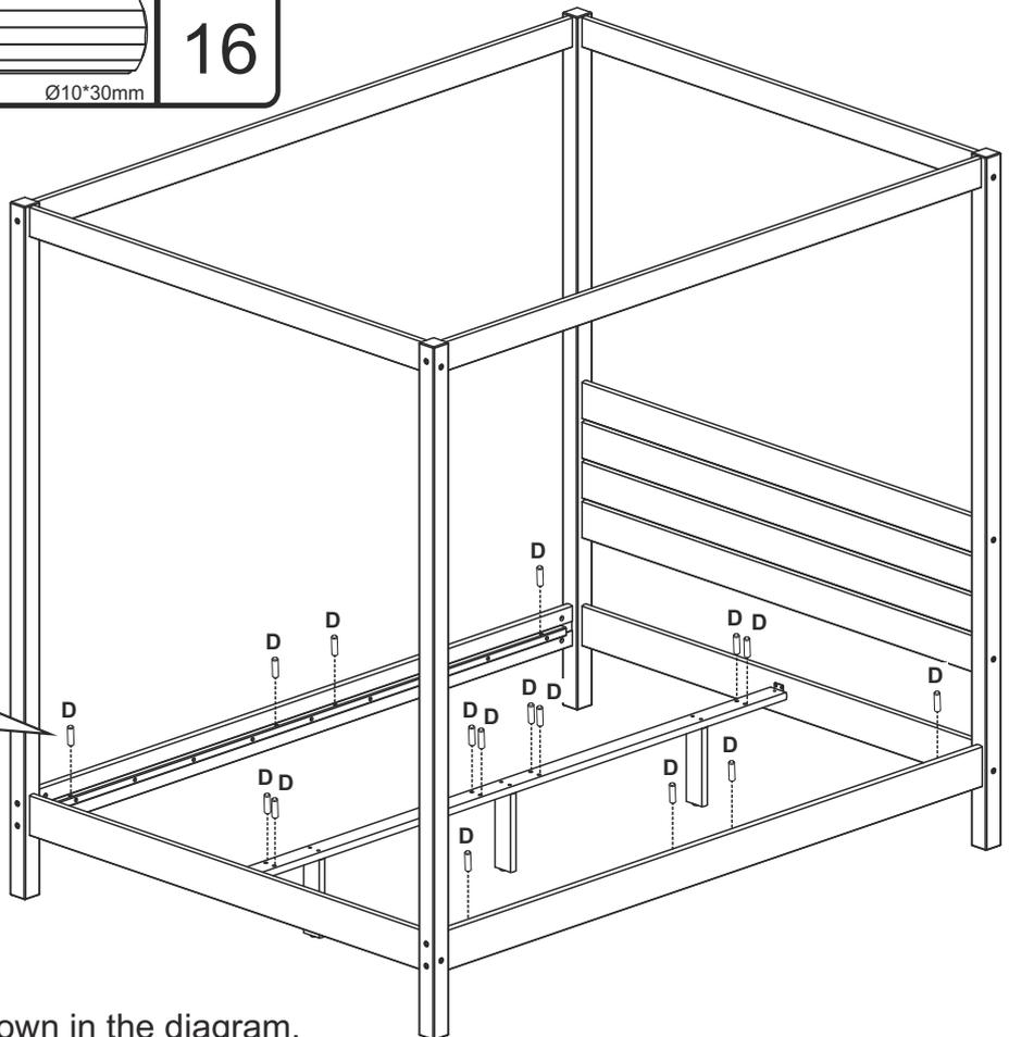
Insert wooden dowel (D) as shown in the diagram.
