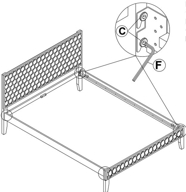
Attach the side rail (P6) to the headboard post (P3) and footboard post (P5) using hardware:
