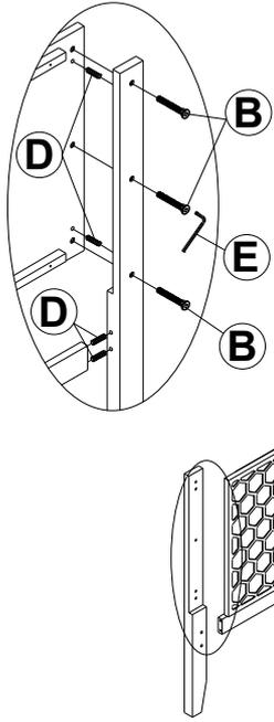
Attach the headboard post (P3) to the headboard panel (P1) and headboard bottom rail (P2) using hardware:
