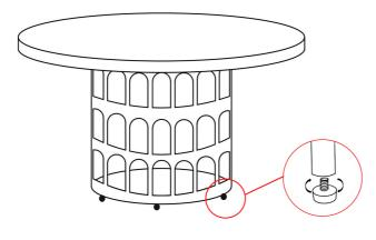
Tip for leveling of product: When the product rests on an uneven floor suface it will appear to be unbalanced to aid in levelling, try adjusting the levelers located on the bottom of each foot.
