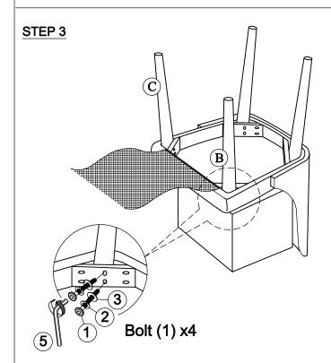
Do not tighten bolt until completely assembled.
