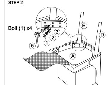
Do not tighten bolt until completely assembled.
