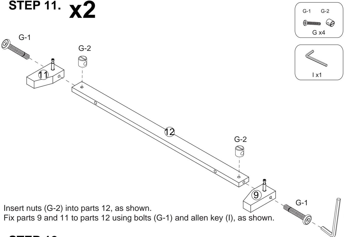
Insert nuts (G-2) into parts 12, as shown.
