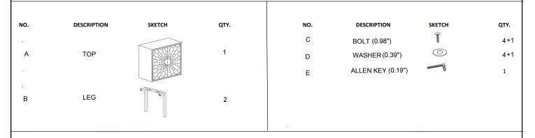
STEP: - Unpacked the legs and tighten the legs with all bolts and washers.
