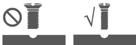
**6** Make sure you understand which hardware will be used on each step. Using the wrong size of screw, bolt or pin might strip the threads or cause damage to the part in which it is being used.
