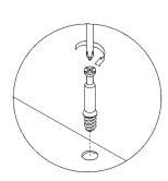
2. Place the other panel over the panel with the bolt, then insert the cam lock to join the bolt's head. If the cam lock does not want to enter, check its proper alignment. There might be a very small gap between the panels which is normal.
