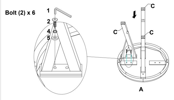
STEP 2: Using the Allen key to tighten all bolts.
