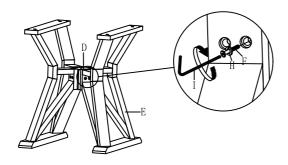
Step 4: Attach Table Leg Top Support B with Table Top A by insert (I,H & G).
