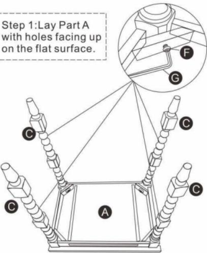
Step 2: Parts C screw to Part A using Parts F and Part G.
