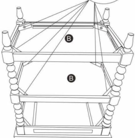
Step 4: Part E screws to Part D and then insert Part D into Part A.
