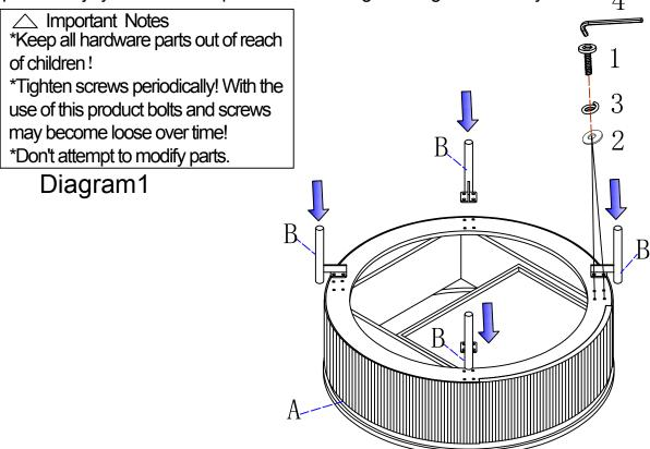
Begin by placing the table upside down on a smooth surface please make sure the surface is not abrasive.
