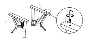
Step 2: Attach Table Leg Top Support B with Table Leg E by insert (I,H & G).
