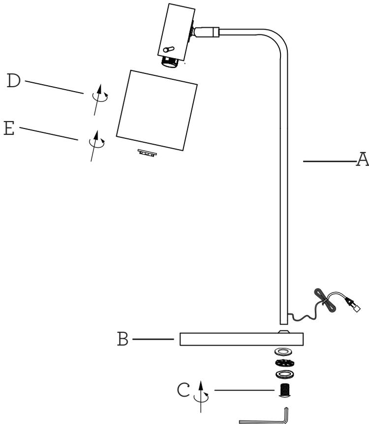
1. Insert pole (A) into base (B). From the bottom of the base, place 3 metal pieces in the order shown on the diagram onto the pole and screw on screw nut (F) using the allen wrench. Make sure to fasten tightly so the lamp is sturdy. When you turn the lamp right-side up, be sure the shade is facing forward so that it hangs over the base.
