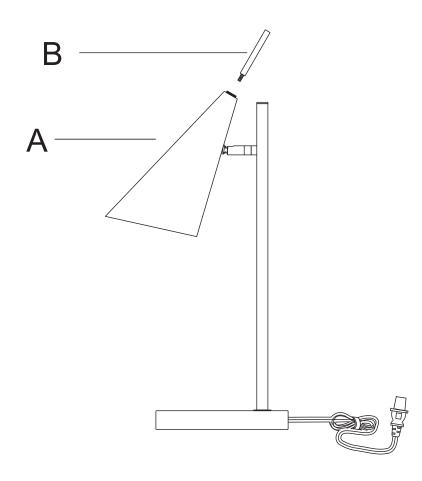
1.Screw shade accent (B) clockwise into shade(A) to tighten.
