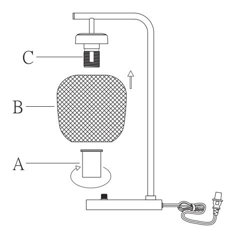
Socket ring (A) comes pre-assembled to the socket (C). Before assembling the shade, please unscrew this socket ring (A). Set shade (B) onto socket (C) and tighten clockwise with socket ring(A) to secure shade.
