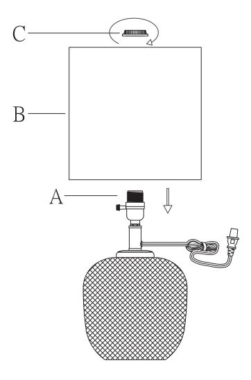
Socket ring (C) comes pre-assembled to the socket (A). Before assembling the shade, please unscrew this socket ring (C). Set shade (B) onto socket (A) and tighten clockwise with socket ring(C) to secure shade.
