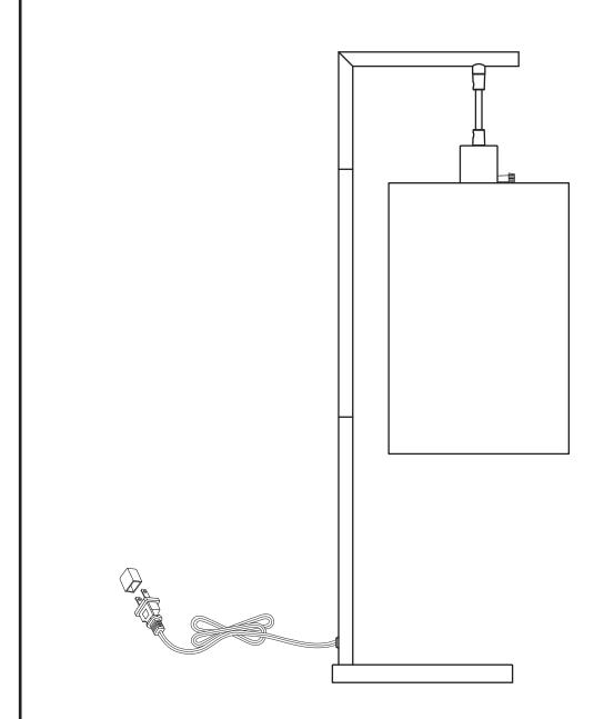
1. Screw tube (A), (B) and (C) until tight. You may need to pull out excess cord gently from the cord outlet of tube (C).
