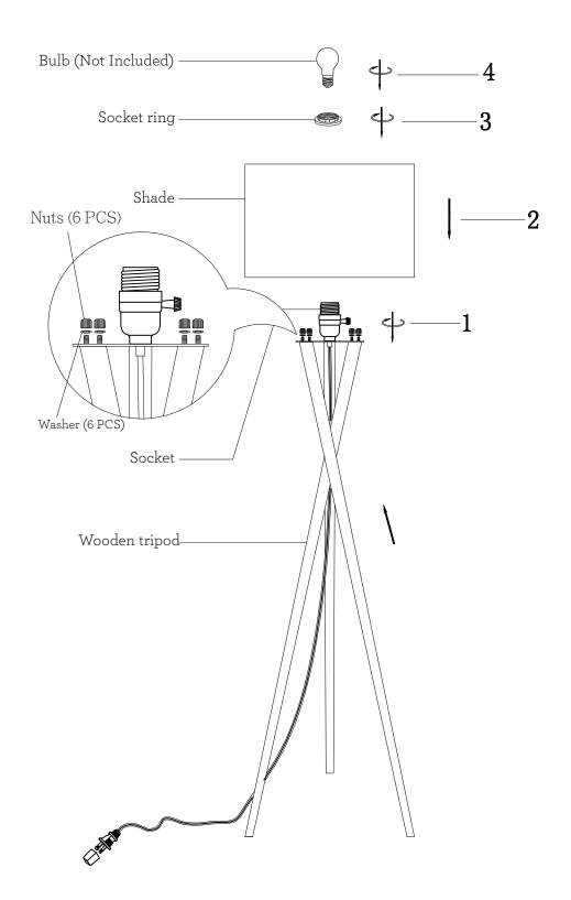
1.Unscrew the nuts from the wood and take off the washers. Set the wooden leg onto the socket plate and then put the washers onto the screws again and screw the nuts on clockwise to tighten.
