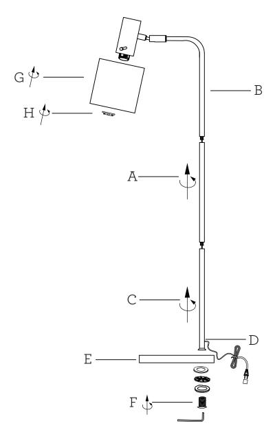
1.Screw pole(A) clockwise onto pole(B) to tighten.
