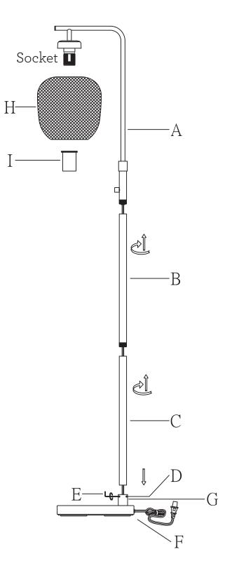
1. Screw pole (B) clockwise onto part (A) to tighten.
