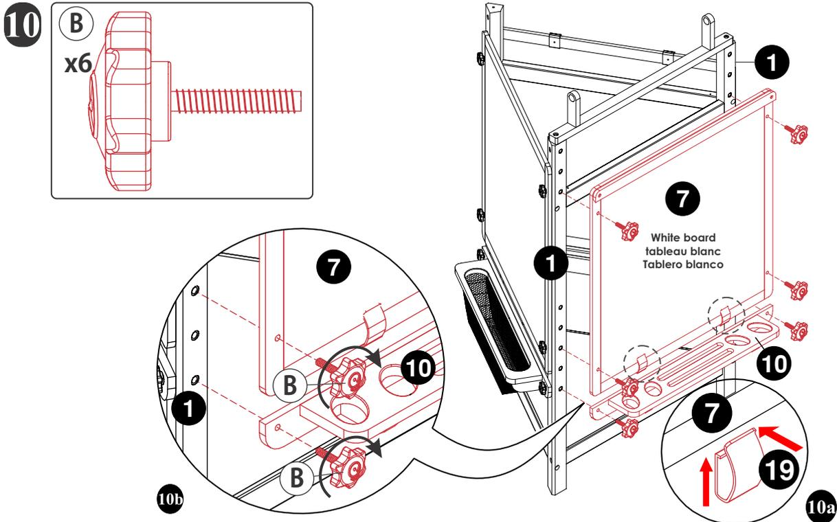
**Note/Remarque/Nota:** Do not tighten all bolts until all four bolts are in place to help with alignment.
