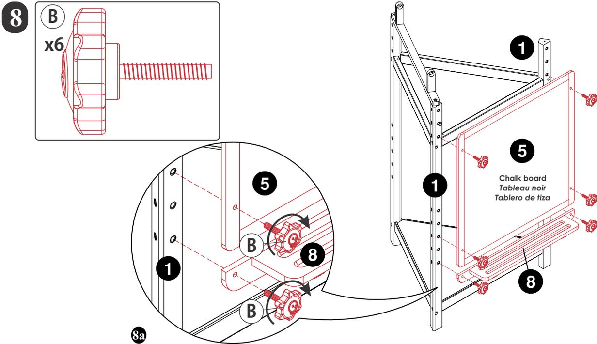
**Note/Remarque/Nota:** Do not tighten all bolts until all four bolts are in place to help with alignment.
