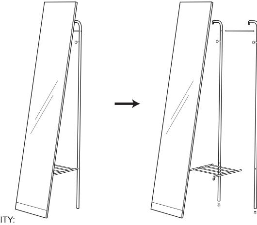
WEIGHT CAPACITY: MAXIMUM LOAD FOR EACH HOOK IS 3KGS(6.6LBS). WIRE SHELF CAN NOT EXCEED 5KGS (11LBS).
